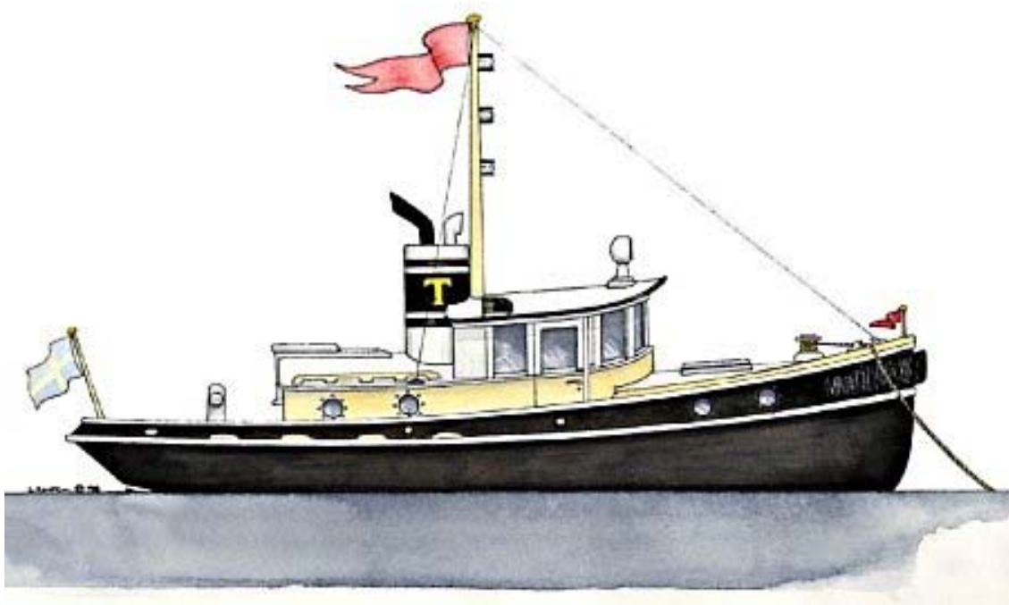
A design for construction in steel - the 32' tug-yacht Terrier
